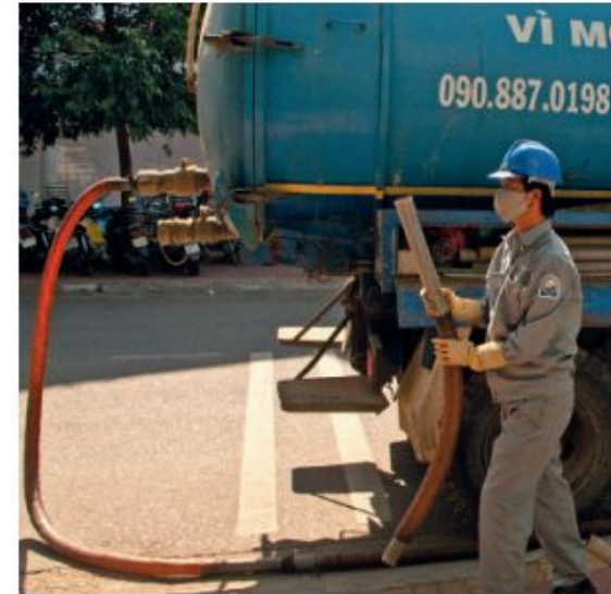
Figure 4.12 Example of correct method where the hose is easy and quick to assemble (photo: Linda Strande).
