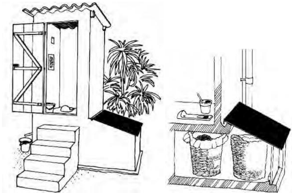
Eco Toilet with Solar heated processing Chamber and Moveable Basket Feces Containers
