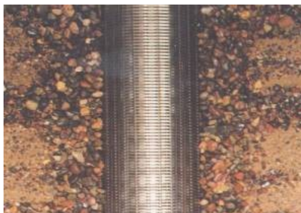
Figure 14: A natural screen develops around a slotted pipe
