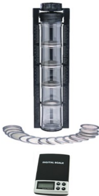
Photo 9: Keck sand shaker and scales
